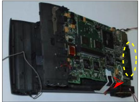
**⚠** Do not touch the Contacts neither on the cable nor on the board. The Stylus-Recognition will be irreparably damaged in this case.
